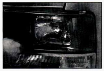
Remove the four screws from the headlamp bezel.
